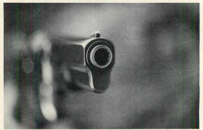
Front view illustrates lack of recoil spring plunger similar to P-35 Browning. Solid front of slide where plunger would normally be aids in simplifying disassembly — fewer parts to deal with.
